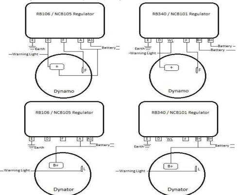
The NCB133 model 340 now replaces the old model RB310 type regulators. There are some physical differences in the two units but they are interchangeable. Model 310 was supplied with three terminal connections; B, F and D. It's replacement model RB340 has five; E, D, WL, F and B.
