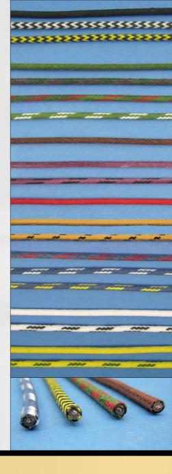
Braided cable is an authentic replacement cable for older vehicles such as classic and vintage cars. Manufactured by braiding modern PVC cable and then lacquering. The cable therefore looks like the original but has the electrical and mechanical properties of modern cable.
